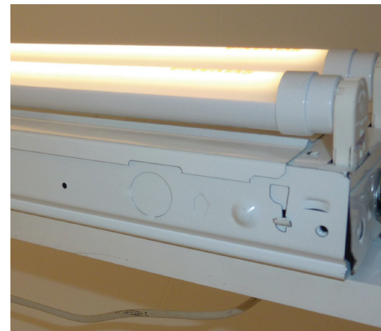
LED T8 in testing chamber. Note the light only comes out of the top.
