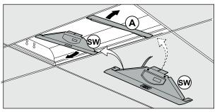
Installing Controls Platform: Install one side panel (A) and one EvoKit SpaceWise panel (SW)
