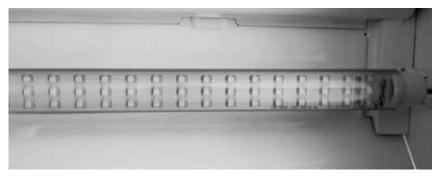
potentially being unsafe, you should check with your insurance company before proceeding. So, even though the LED T8 product may be UL listed, the luminaire that it is being installed into was not rated for line voltage to the sockets.
