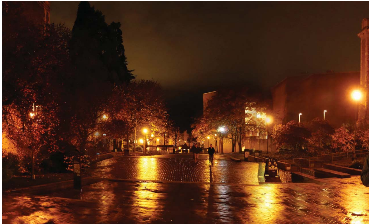
Figure 5. Traditionally, high pressure sodium sources have been used to light pedestrian-oriented landscapes, with characteristic warm color temperatures and low color rendering properties.
