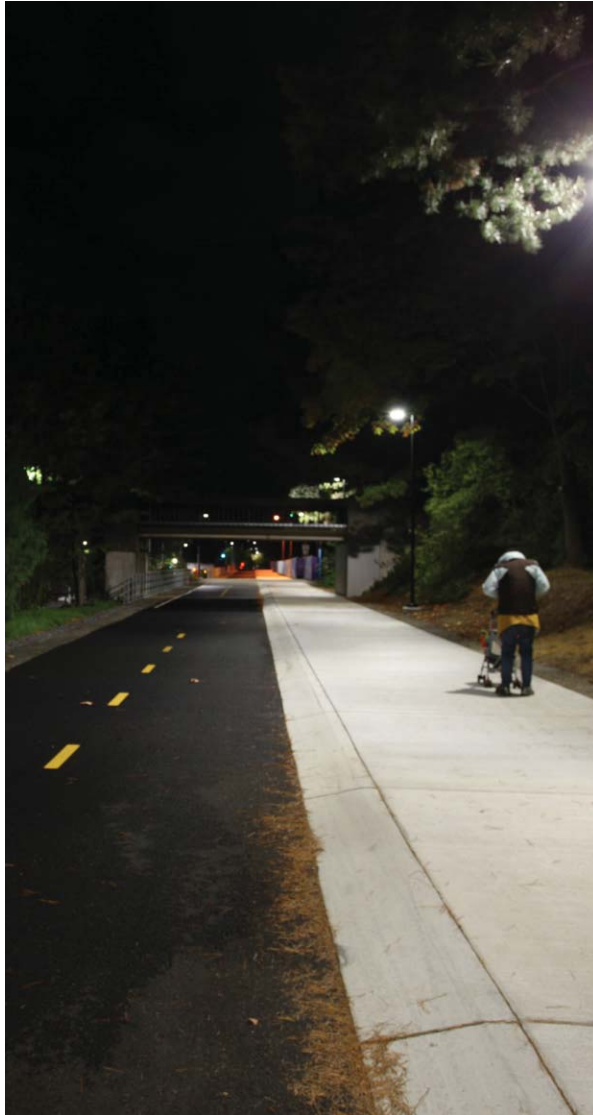
Figure 18. The Burke-Gilman Trail along NE Pacific St. uses landscape material surfaces with different reflectances to delineate nighttime circulation routes for different modes.
