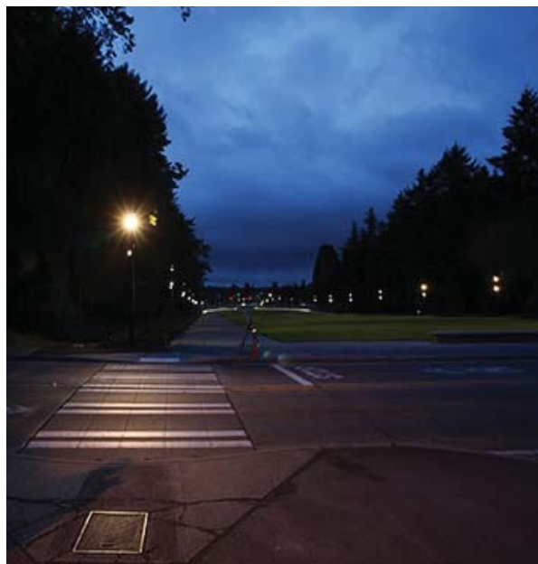
Figure 7. Illuminance measures the light that is emitted from a source, while luminance reveals light conditions as the eye perceives them. This HDR analysis of a Rainier Vista crosswalk illustrates the luminance of this space.
