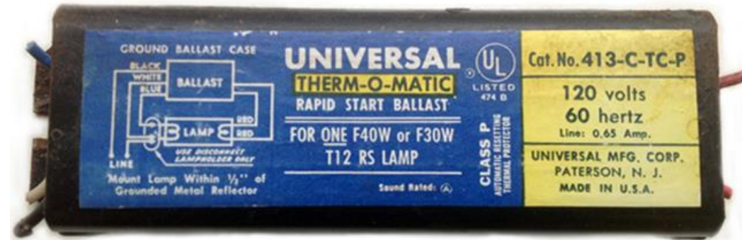
A typical pre-1979 PCB-containing fluorescent light ballast (FLB)
