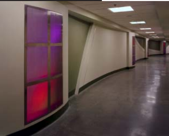
Above: The Evergreen Medical Center corridor uses color changing lighting to add visual interest in an ordinarily pedestrian space. Ms Enlow conducted several mockups at the LDL as part of the development of the design. Photo courtesy Sparling Electrical Engineering.
